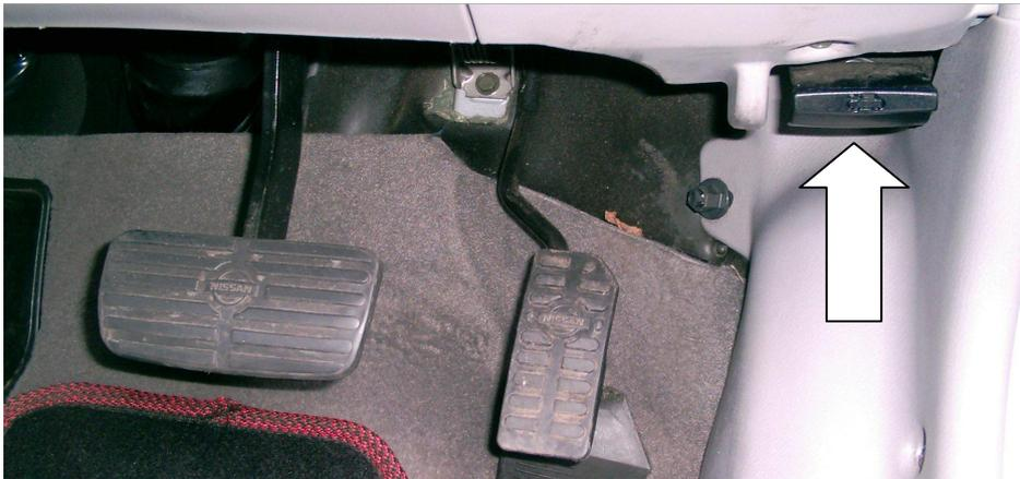
**Step 1:** From inside the car pull the handle (arrowed) towards you.
